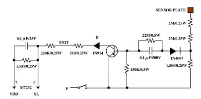
All switching and dimming functions can also be implemented by utilizing the SL input. This can be done by either a mechanical switch or the electronic switch in conjunction with a Sensing Plate. When the plate is touched, a logic high level is generated at the EXTENSION terminal for both half cycle of the line frequency.
